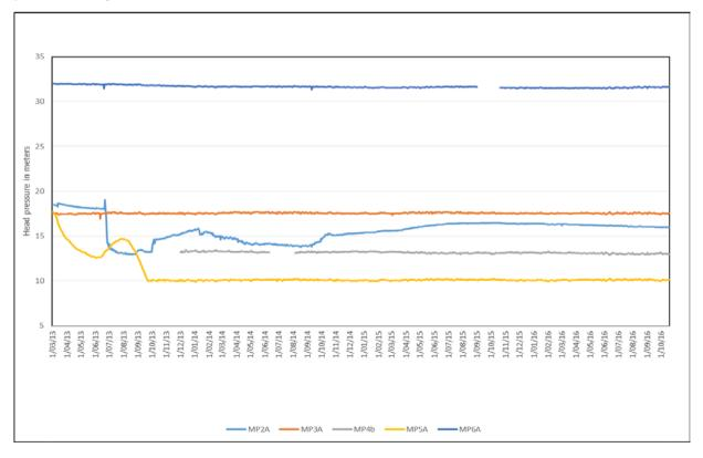
Figure 2 Rocglen VW Piezometers Ground Water Head Pressure
